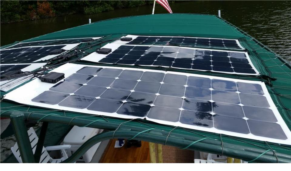
Six 100 Watt Semi-flexible Panels Sewn On
