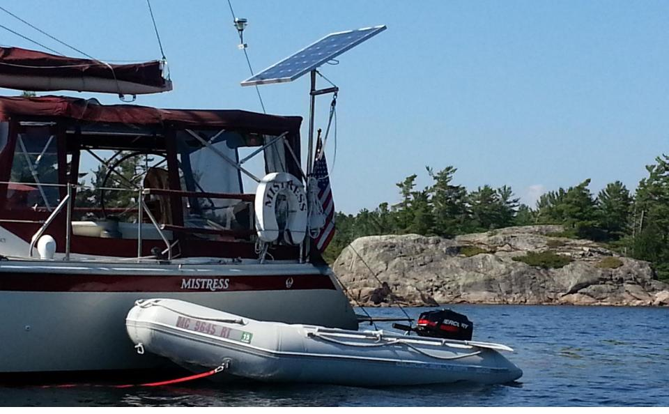
175 Watt Panel on a Pole with Outboard Motor Crane Tilt and Rotate
