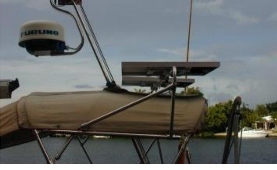
Two Panels on a Bimini Mounted Frame
