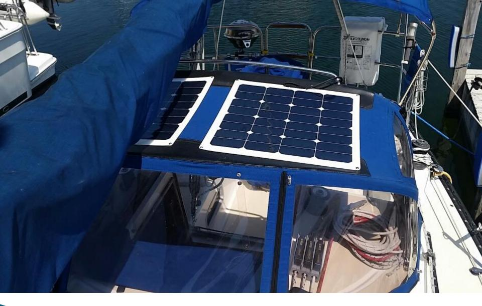
Two 50 Watt Semi-flexible Panels Bolted On
