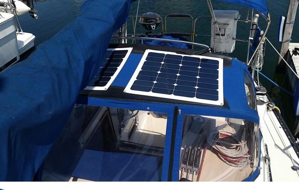
Two 50 Watt Semi-flexible Panels Bolted On
