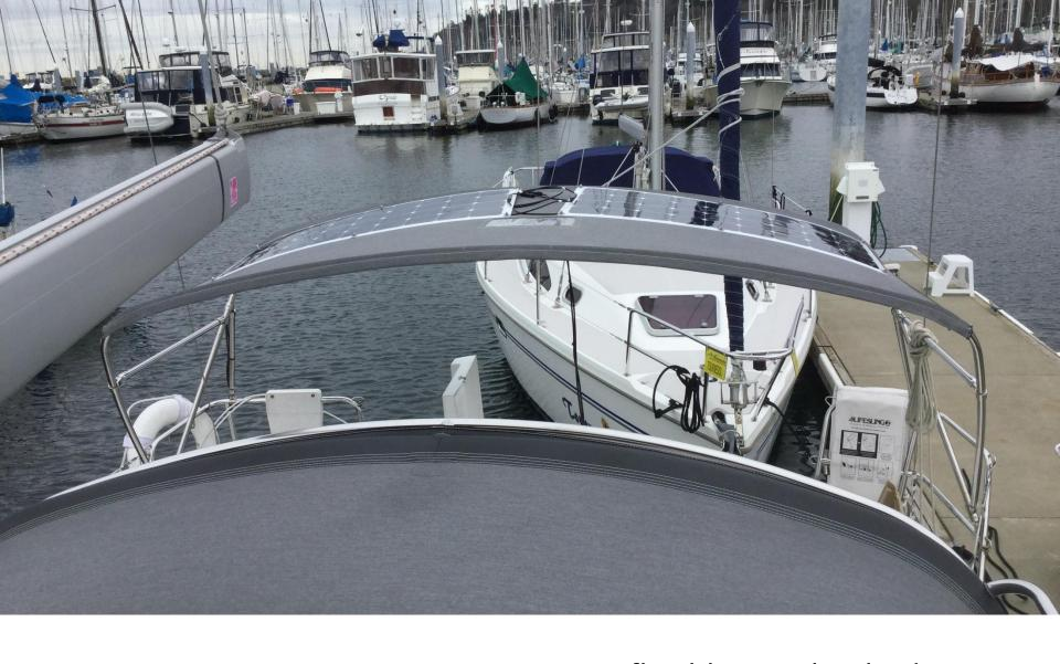
110 Watt Semi-flexible Panel Bolted On
