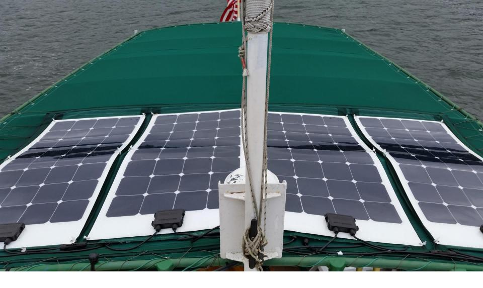
Four 100 Watt Semi-flexible Panels Sewn On
