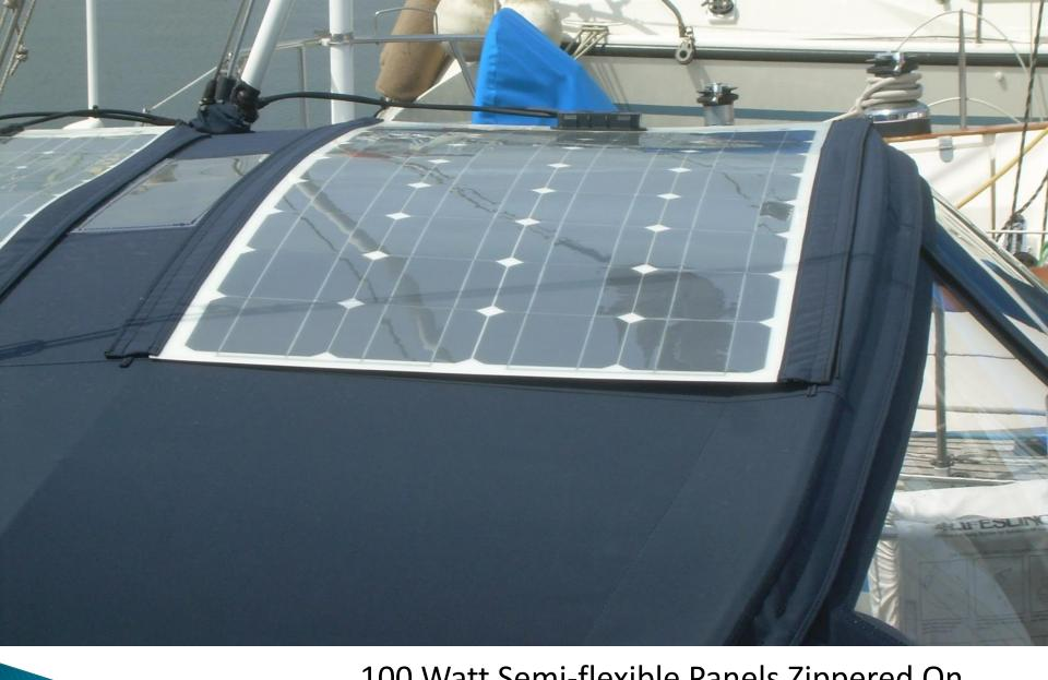
100 Watt Semi-flexible Panels Zippered On
