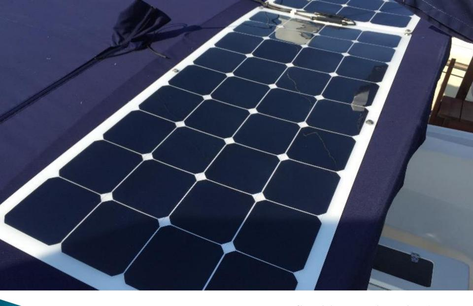
Two 110 Watt Semi-flexible Panels Bolted On
