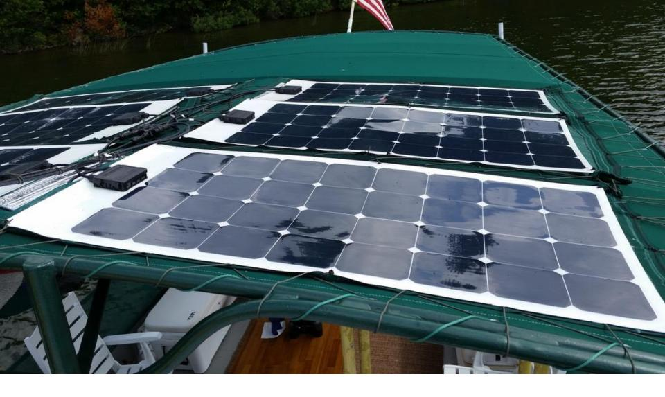
Six 100 Watt Semi-flexible Panels Sewn On
