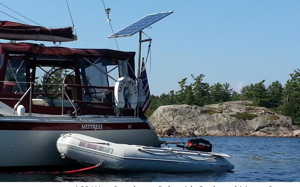
160 Watt Panel on a Pole with Outboard Motor Crane Tilt and Rotate
