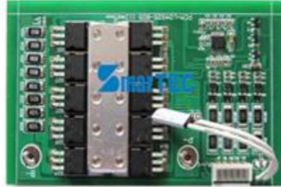
Battery Management System (BMS)
