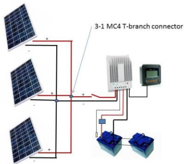
Three Solar Panels Wired in Parallel with One EP Tracer BN MPPT Controller
