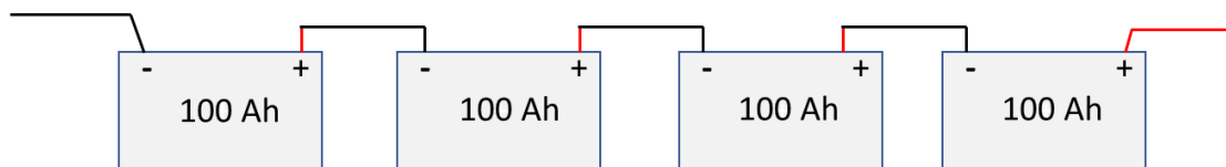
Series - 48 V 100 A Draw Capacity 90 Ah Capacity at 90%
