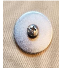
Insert bolt with washer
