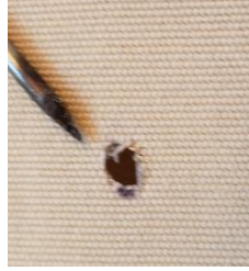
Punch hole with hot tool
