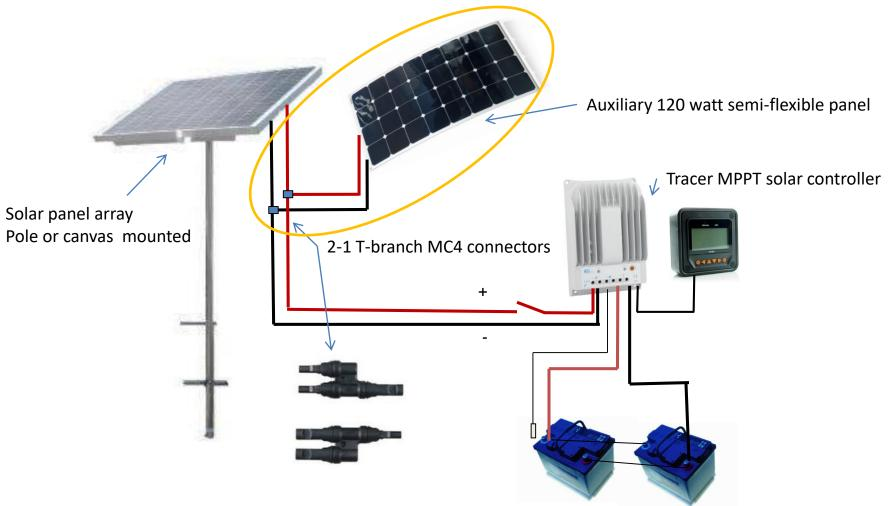
Wiring diagram showing connection of an auxiliary 120 watt solar panel when extra power is needed.
