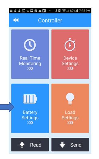
The Controller navigation page has four quadrants. The lower left Battery Settings quadrant is used to set up the battery type and size parameters. Most of these settings can also be defined using the remote or built in meter. The Battery Settings must be used to set up the Lithium battery types.
