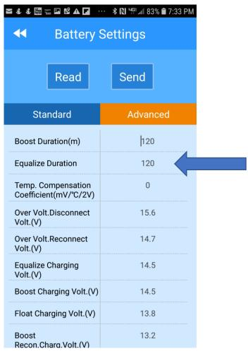
Set each value per the specification of the battery being charged. Equalize Duration should be set to zero for LiFePO4 batteries since this battery technology does not require equalization.
